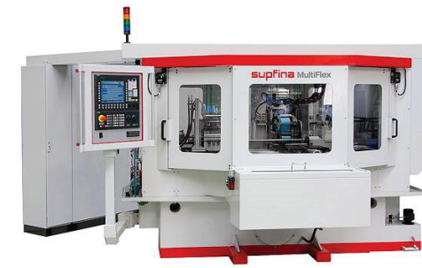
Joonis 3.35 Superviimistlemise masin Supfina MultiFlex (Supfina Grieshaber GmbH & Co. KG)
